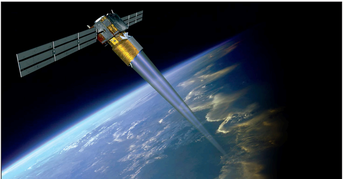
Figure 13. Illustration of Aeolus Doppler Wind Lidar in orbit. (Copyright ESA).
